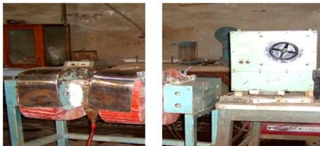
Fig 3. Boxmag rapid WHIMW magnetic separator.
