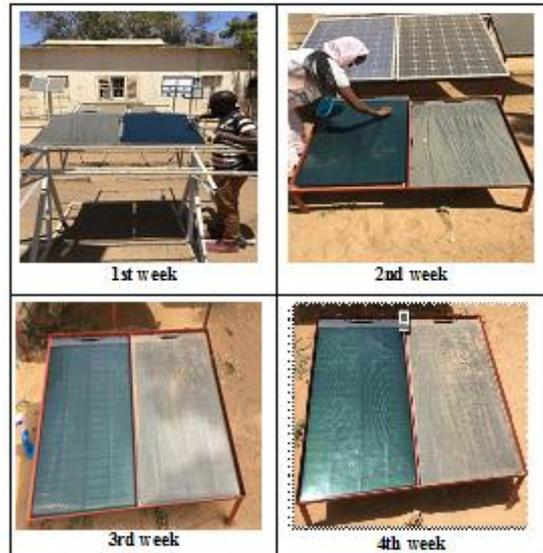
Figure 3. Exposure and weekly monitoring of modules.
