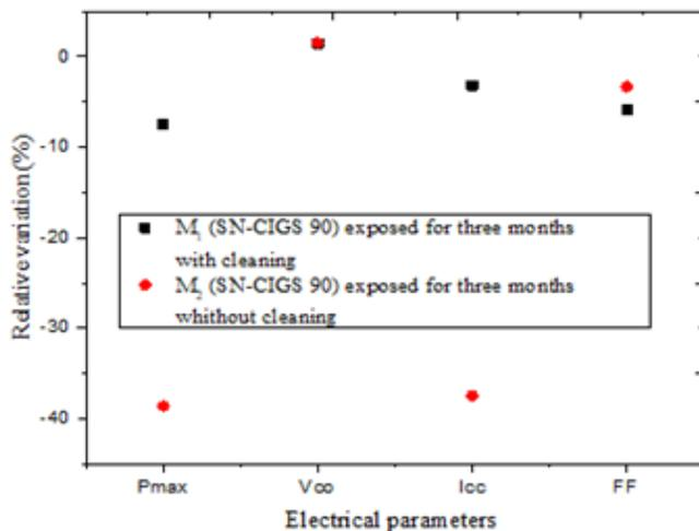
Figure 4. Comparison of the variation rates of the electrical parameters of the two modules after three months of exposure.
