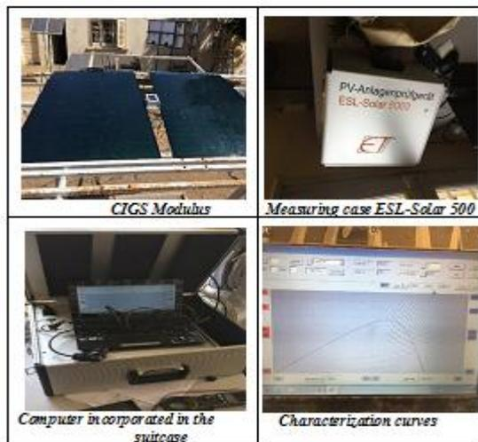
Figure 2. Measurement platform
