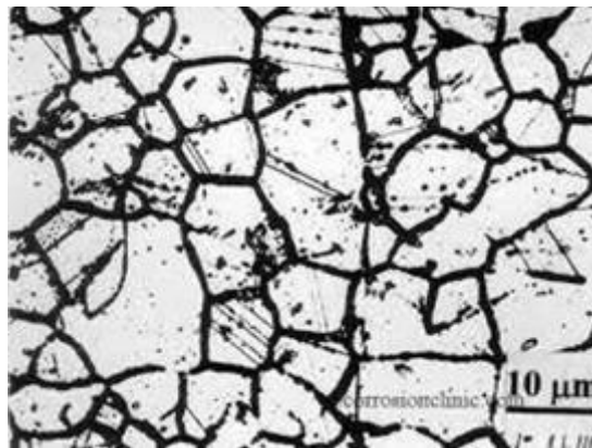
Figure 1.4. Illustration of inter granular corrosion attack
