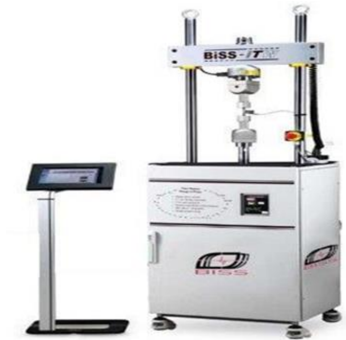
Figure 3.10. Servo hydraulically controlled fatigue testing machine.
