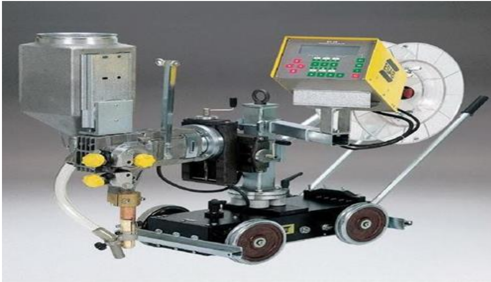
Figure 3.4. Setup of Submerged Arc Welding (SAW)
