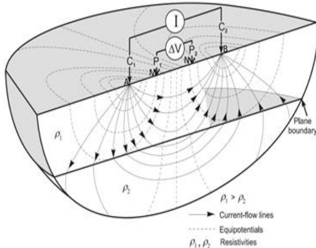
**Fig 4. Principle of VES measurement with a four-electrode array (Adopted from Knodel *et al.* )**
