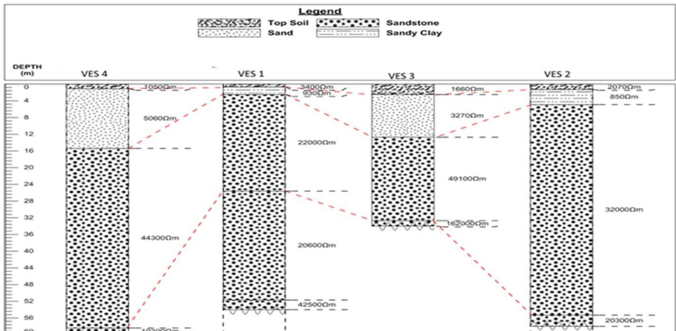
Fig. 12 Geoelectric sections of the VES points.
