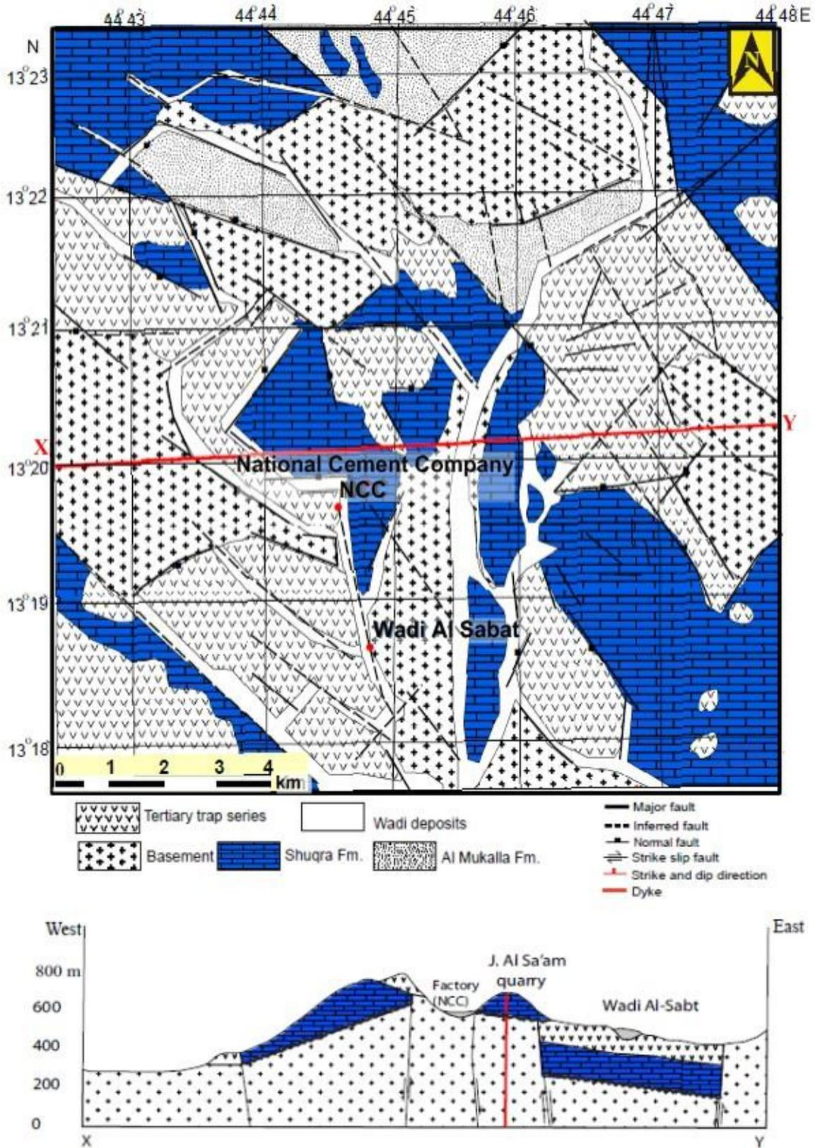
Fig. 6. Detailed geological map of the quarry sites in Lahj area and cross-section from X-Y.
