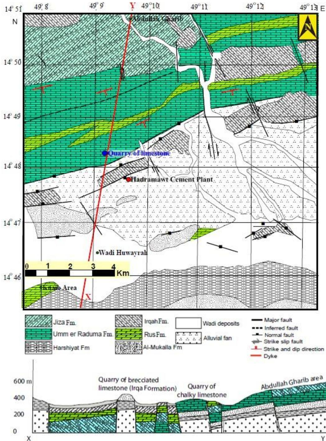
Fig. 7. Detailed geological map of the quarry sites in Al-Mukalla area and cross-section from X-Y.
