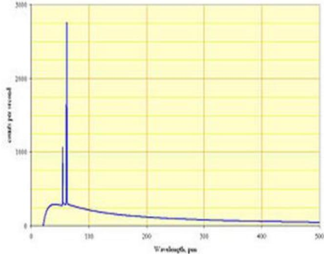
**Spectrum of the X-rays emitted by an X-ray tube with a rhodium target, operated at 60 kV. The smooth, continuous curve is due to bremsstrahlung, and the spikes are characteristic K lines for rhodium atoms.**
