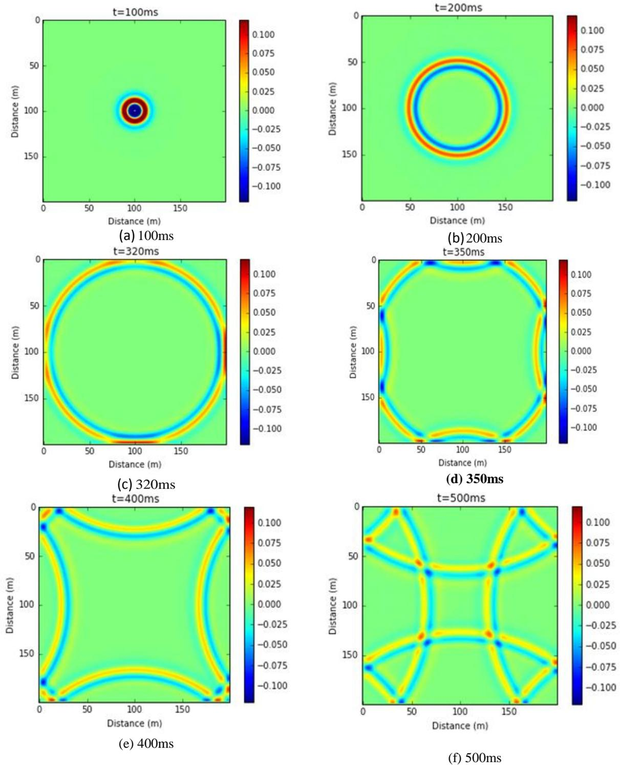
Figure 3. Snapshots of the acoustic wave simulation without PML for a homogeneous model (a)  $100\text{ms}$ , (b)  $200\text{ms}$ , (c)  $320\text{ms}$  (d)  $350\text{ms}$  (e)  $400$  and (f)  $500\text{ms}$ .
