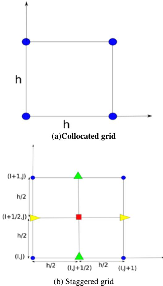
Figure 1. Collocated and staggered finite difference.
