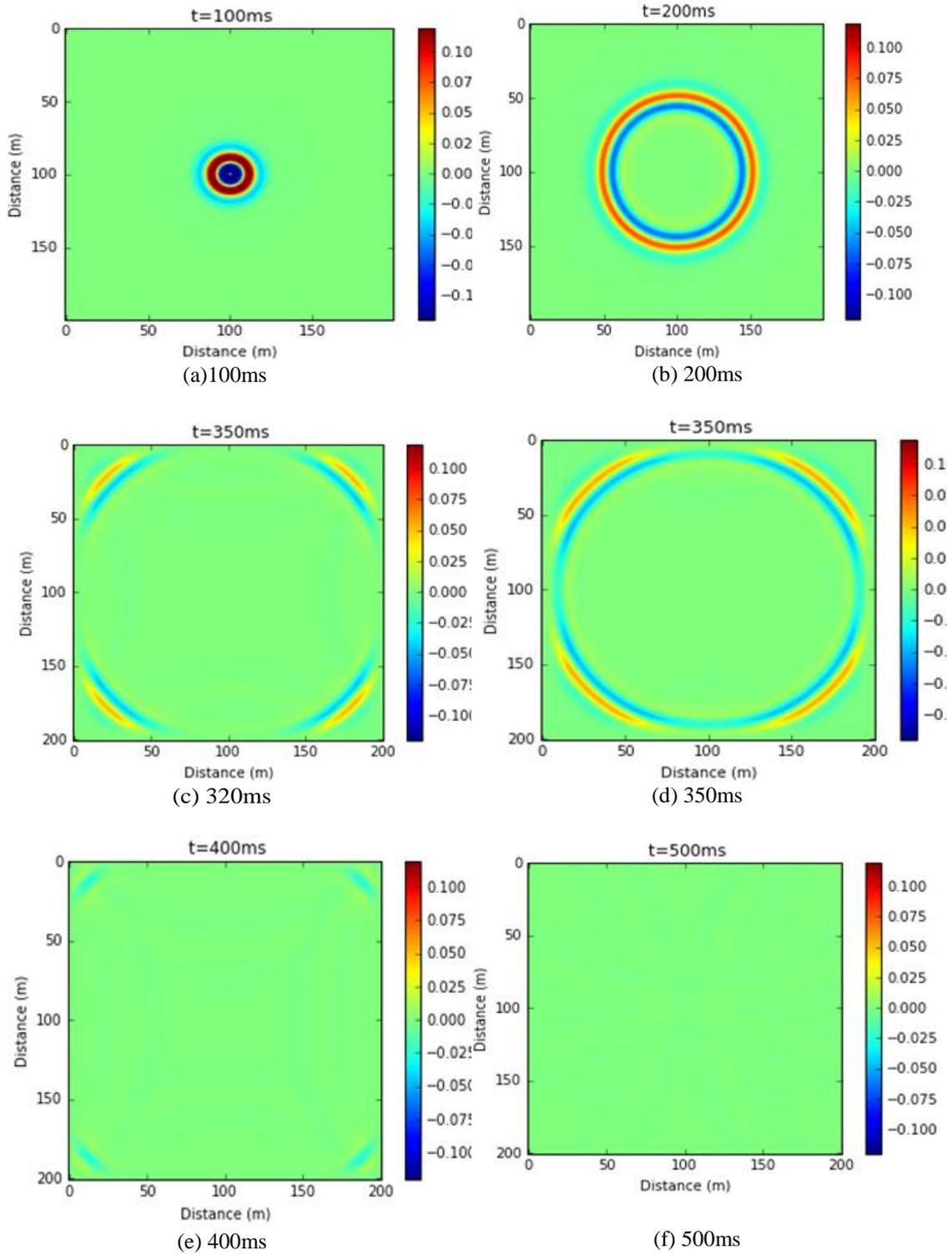
Figure 4. Snapshots of the acoustic wave simulation PML for a homogeneous model (a) 100ms, (b)200ms, (c)320ms (d) 350ms (e) 400 and (f) 500ms.
