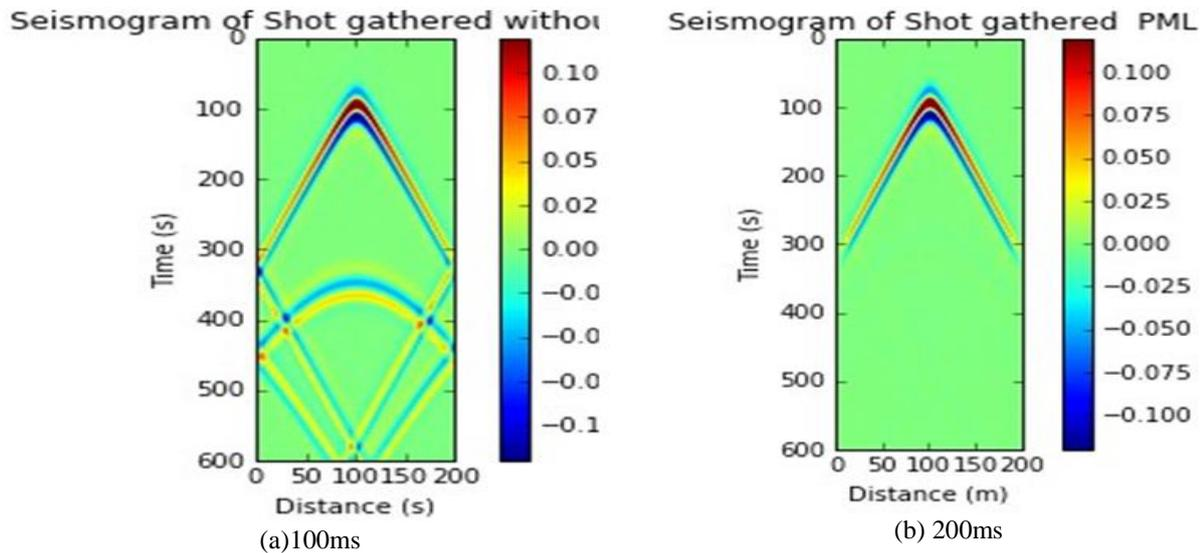
**Figure 5. Shot gather for the acoustic wave equation (a) Without PML and (b) With PML.**
