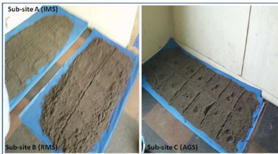
Figure 7. The three different sample bulks showing a grid template of 12 cells created on each sample, from which samples were collected for physicochemical analyses (Adekunle et al., 2015)
