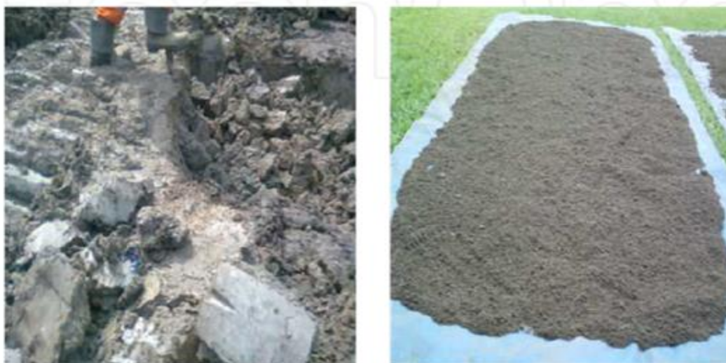
Figure 8. Appearance of the crude-oil-impacted clay soil before and after CNB-Tech treatment (Adekunle et al., 2015)
