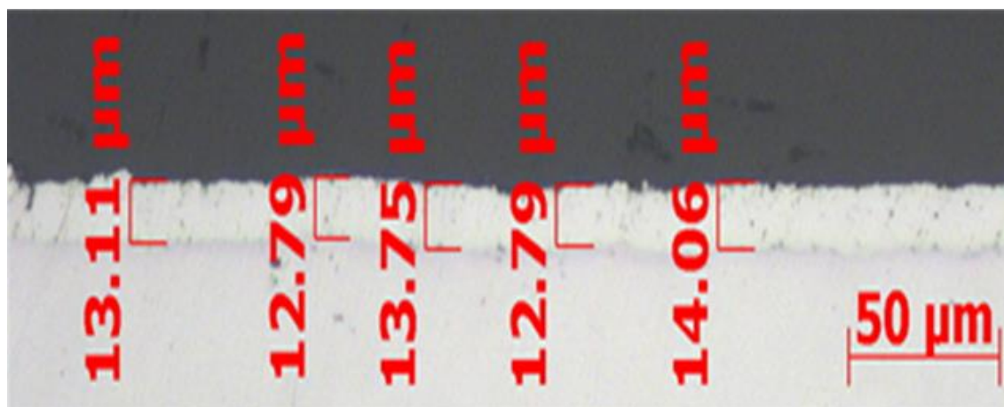
Figure 1. Thickness values of ZnNiSiO 2 coating, with plating time of 20 minutes and plating current density of 3A/dm 2 (measured by Axiovert40MAT)
